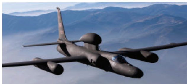
The Raytheon Advanced Synthetic Aperture Radar System-2 (ASARS-2) is a multimode real-time, high-resolution reconnaissance system carried on the U-2 Dragon Lady high-altitude reconnaissance jet.
