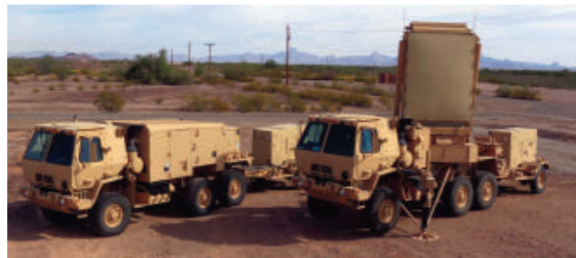
The Lockheed Martin AN/TPQ-53 counter-fire radar detects, classifies, tracks, and pinpoints enemy drones and incoming artillery shells.
