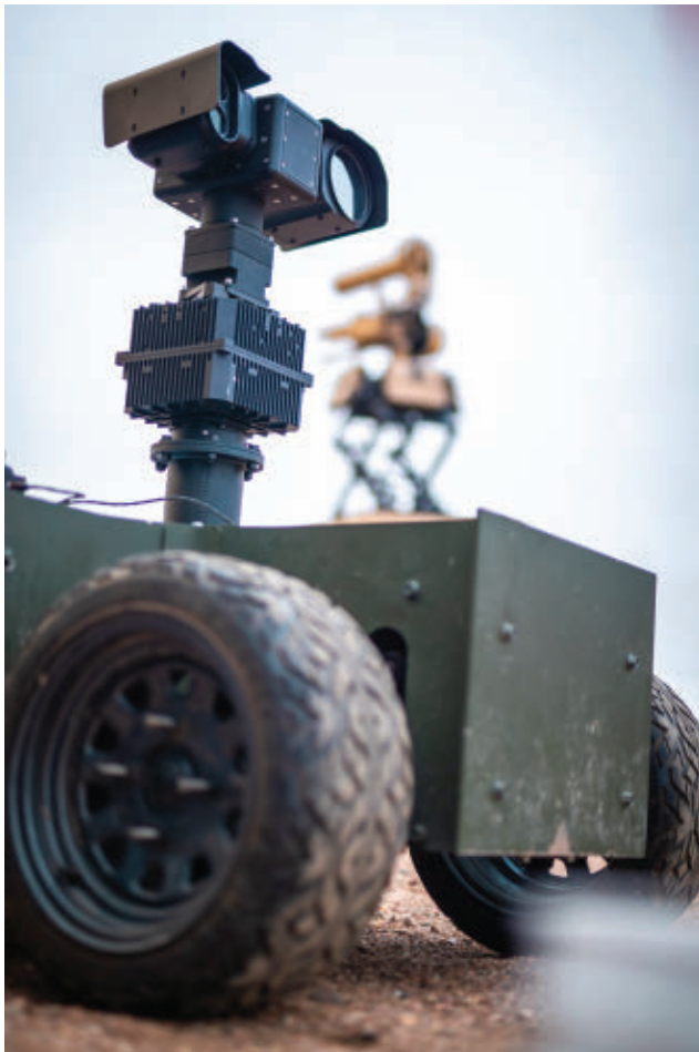
The Multi-Mission Explorer (MDX) counter-unmanned aerial system (C-UAS) from Liteye Systems is a man-portable sensor package that uses 3D radar combined with medium-wave infrared (MWIR) and visible-light sensors.
